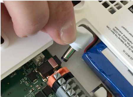
Plug in the power connector
