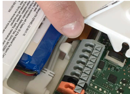
Route the wire behind the retainer clip
